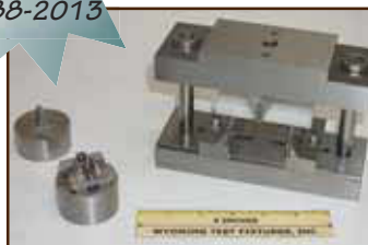
Short Beam Shear ASTM D 2344 Shown with Miniature
