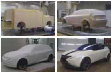
BMW Series1 full scale concept designed and built by Alex Alexiev and his team from the Art Center College of Design in Pasadena, CA. Coastal Enterprises donated Precision Board Plus HDU tooling board for this project.
